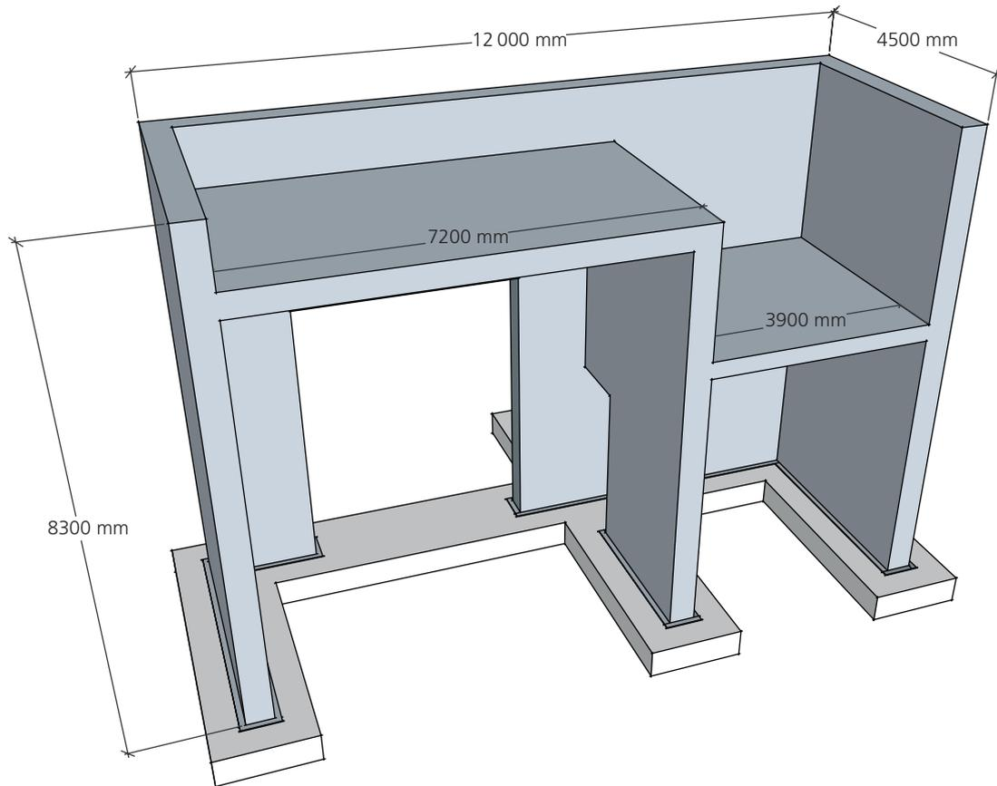
Figure 12. Part of a diesel generator building used to demonstrate construction at full scale
