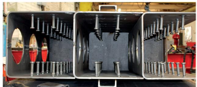
Figure 8. Steel brick-to-steel brick weld detail
