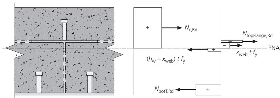
Figure 7. Stress blocks of a case where the PNA is within the top tee
