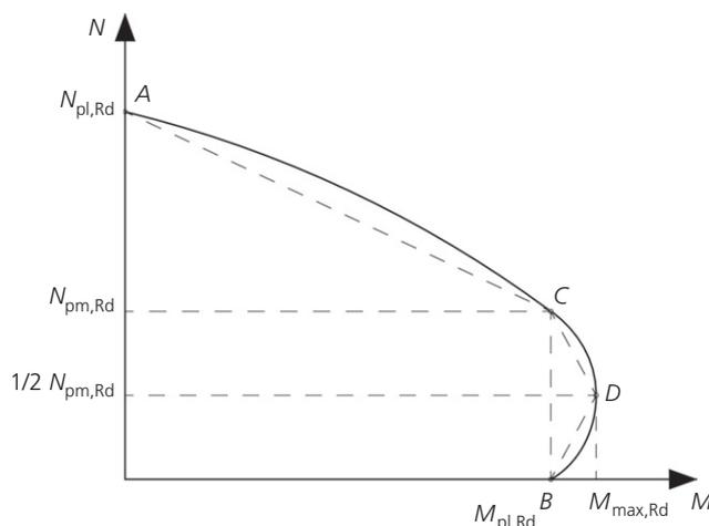
Figure 5. Interaction curve for combined compression and bending with points A to D
