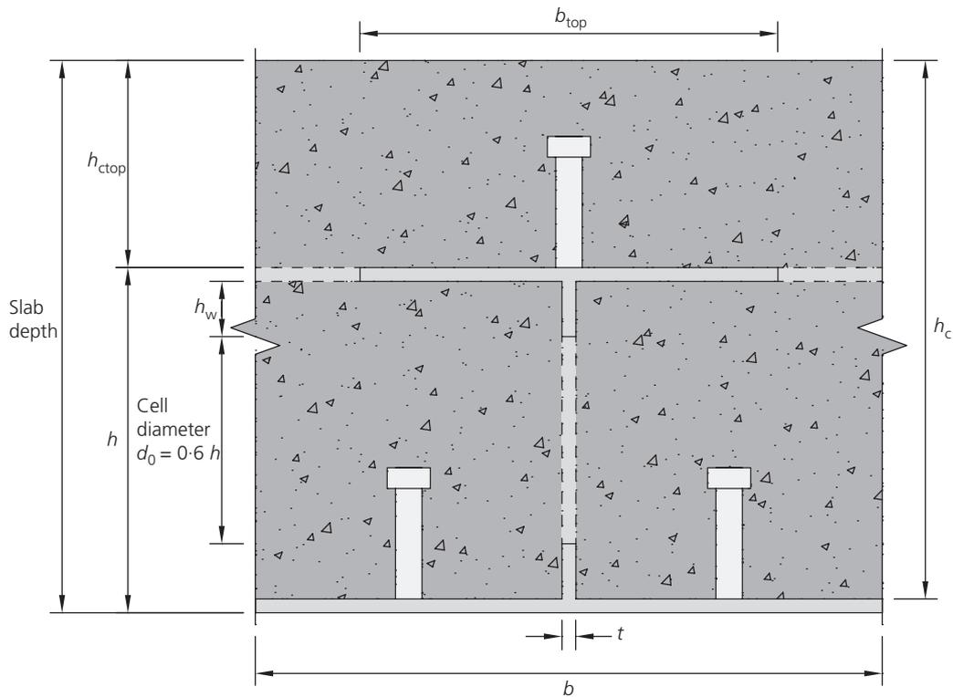
Figure 6. Composite horizontal steel brick member notation
