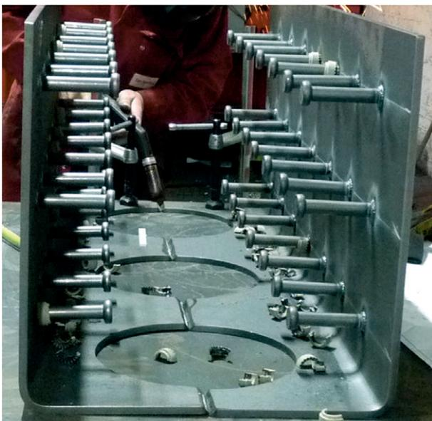
Figure 2. Steel brick concept
