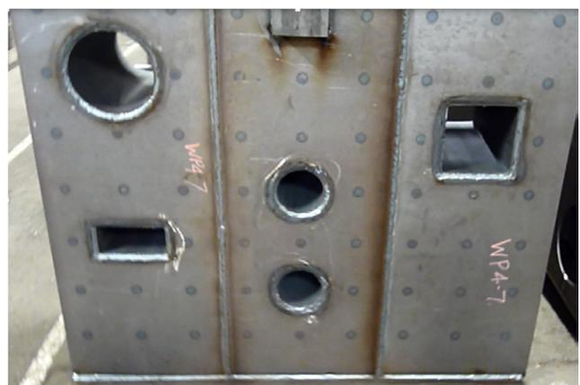
Figure 9. Steel bricks with penetration details
