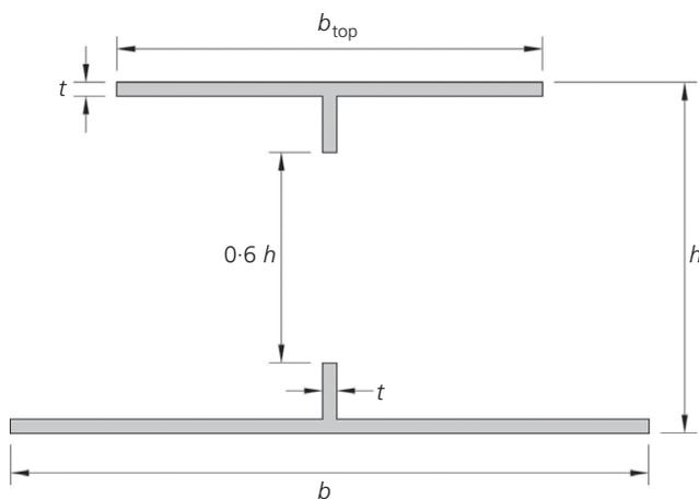
Figure 4. Horizontal steel brick member modelled as an asymmetric I-section
